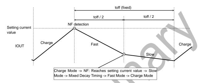
If the output current is zero-detected during OFF time, the output becomes High impedance.
